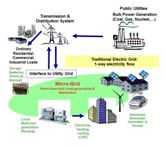
Figure 29 - Example of Microgrid Structure
