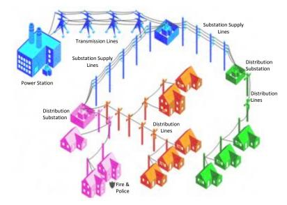
Figure 8 - Illustration of Power System Components
