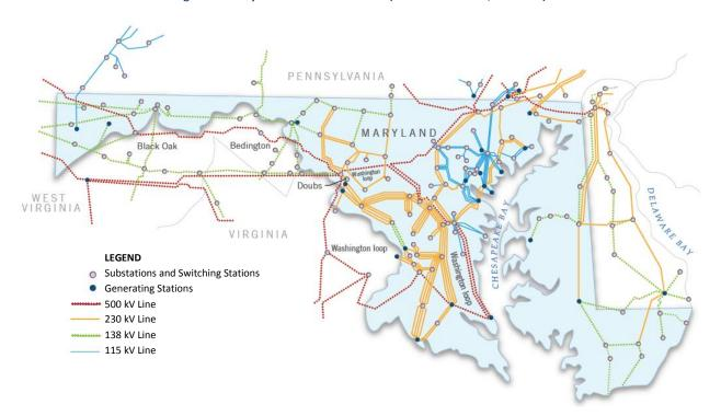
Figure 4 - Maryland Transmission Lines (Greater Than 115,000 Volts)
